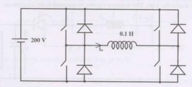
The inverter is operated at 50 Hz in 1800 square wave mode. Assume that the load current does not have any dc component. The peak value of the inductor current io will be
