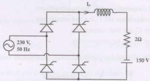
Assume that the load inductance is sufficient to ensure continuous and ripple free load current. The firing angle of the bridge for a load current of  $I_0 = 10$  A will be
