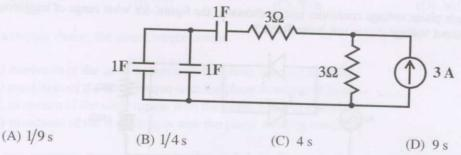
Q.22 The resonant frequency for the given circuit will be
