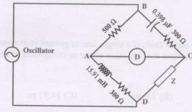
If the bridge is balanced for oscillator frequency f = 2 kHz, then the impedance Z will be
