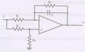
Q.80 If  $R_1 = R_2 = R_A$  and  $R_3 = R_4 = R_B$ , the circuit acts as a
