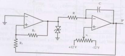
If the voltage  $v_i$  is made +2.5V, the voltage waveform at point 'P' will become
