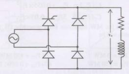
If the firing pulses are suddenly removed, the steady state voltage (v<sub>o</sub>) waveform of the converter will become
