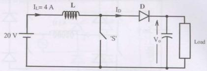
The average voltage across the load and the average current through the diode will respectively be
