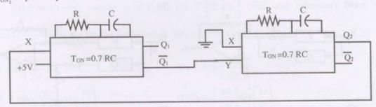
The frequency and the duty cycle of the signal at Q1 will respectively be
